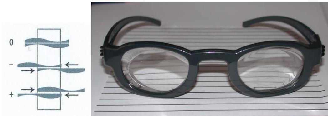
*Figure 4. (Left) The principle of the Alvarez lens (Right) The Focusspec. In this design, the lateral translation of the components of each Alvarez lens is achieved by rotating the helical gears on each side of the frame. Note the different magnifications given by the two lenses, which have been set to powers corresponding to the two ends of the available range (+0.5 and +4.5D). Spectacles with power range -1.0 to -5.0D are also available.*
